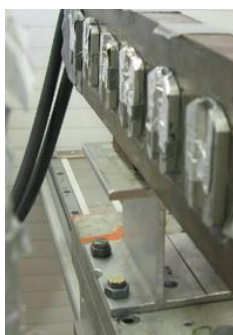
Figure 9. 6 position sample holder with temperature regulation
